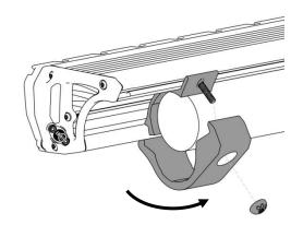
5. Lightly fasten light bar to tube by attaching supplied ARB M6 security nuts to T-bolts. Adjust rotation of light bar on tube to appropriate position and tighten security nuts using security key provided to 9 Nm / 80 lb-in.
